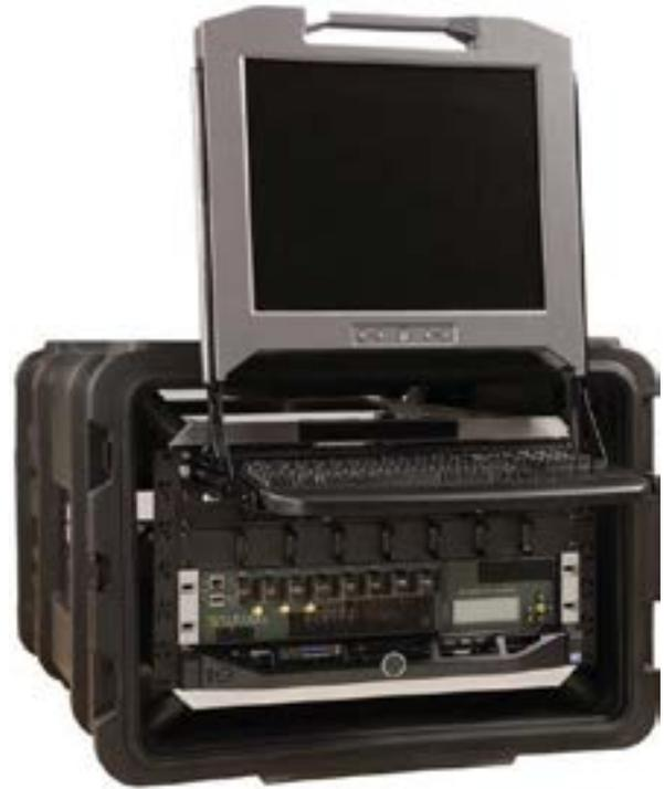
The Virtana portable Performance Assessment Kit (PAK) is an integrated mobile unit that includes everything required to identify the root causes of Storage NAS or SAN performance and availability problems. This mobile unit can be easily moved from Virtana and between data centers due to its rugged, integrated design.
