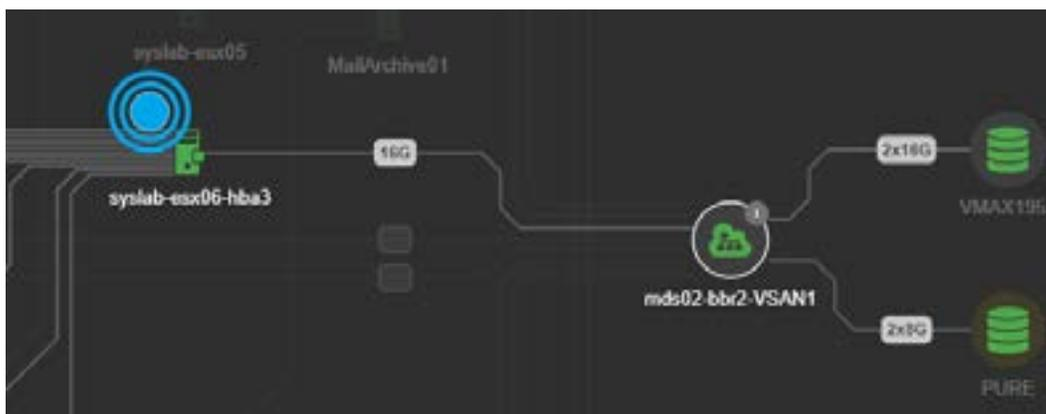
The VirtualWisdom screenshots above show extracts of various performance findings that ultimately reveal the root cause – a “Flow Control” issue in the environment. Virtana performance experts leverage VirtualWisdom analytics to discover the correlation between Storage Port PURE-CT0-FC1 % Time at Zero Receive Buffer Credit metric and HBA Port syslab-esx06-hba3 Read Payload Rate metric. The flow control issue was caused by a speed mismatch between the HBA port (16G) and the storage port (8G).
